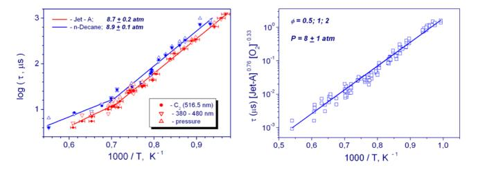
Fig. 2. Ignition times versus reciprocal post-shock temperature behind reflected shock wave in *Jet-A* and *n-Decane* stoichiometric mixtures.
